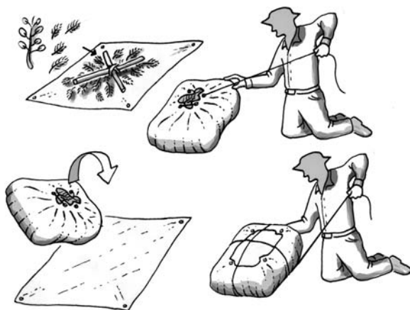
Figure 11-4: Making a trapped-air raft to cross rivers and streams.
